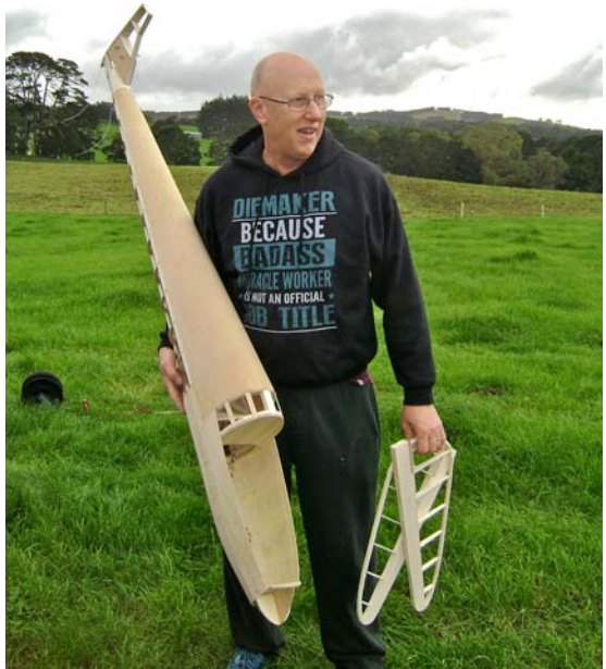
Upper: Stuart Ward at Aka Aka with his next glider under construction. The fuselage is planked with 0.8mm ply. Lower: Visitor Keri Sergison with Stuart launching Keri's Sophisticated Lady using a Hi-start bungee..
